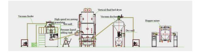
Production Process Flow For The Newly-Designed Solid Dosage Production Line
